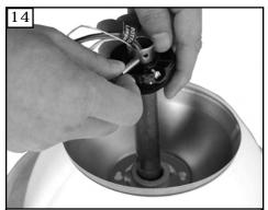
Install half ball on downrod and slide pin into hole in downrod. Then raise half ball so that pin fits in notches in half ball.
